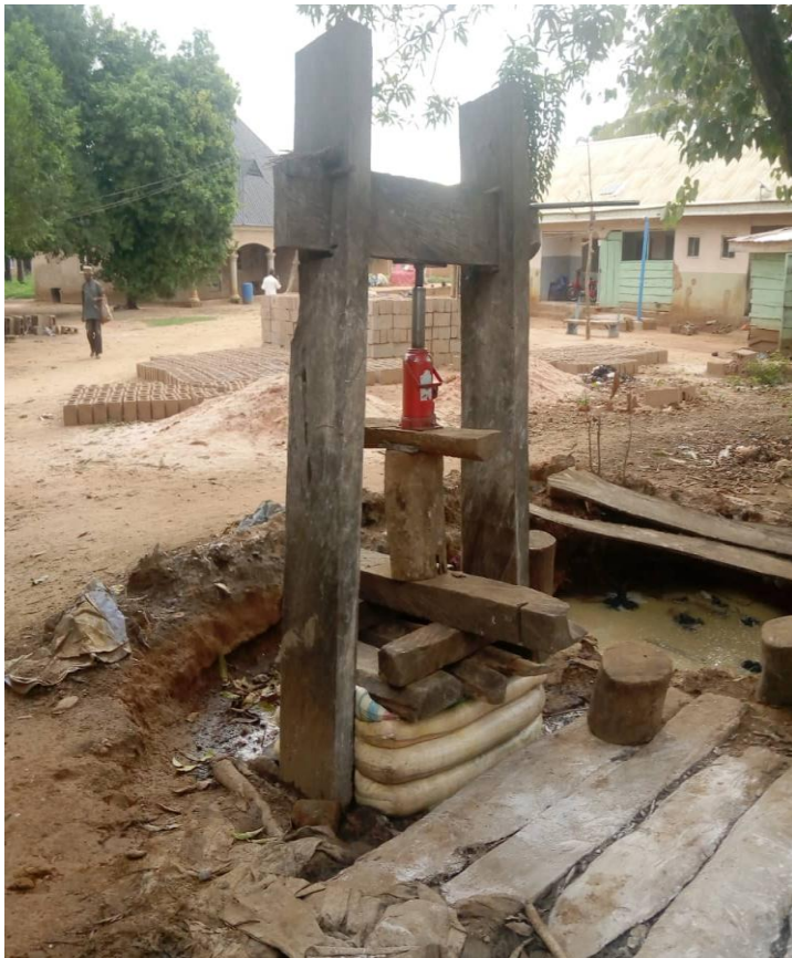
Picture 5: Dewatering/Pressing of mash with a hydraulic Jack
