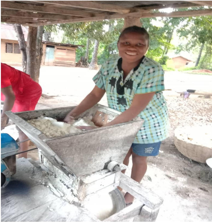
Picture 3: Grinding of cassava tubers into mash.
