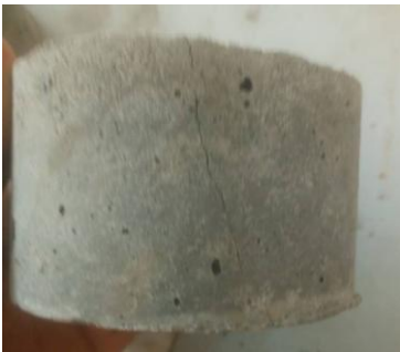
c. Cracked specimen
